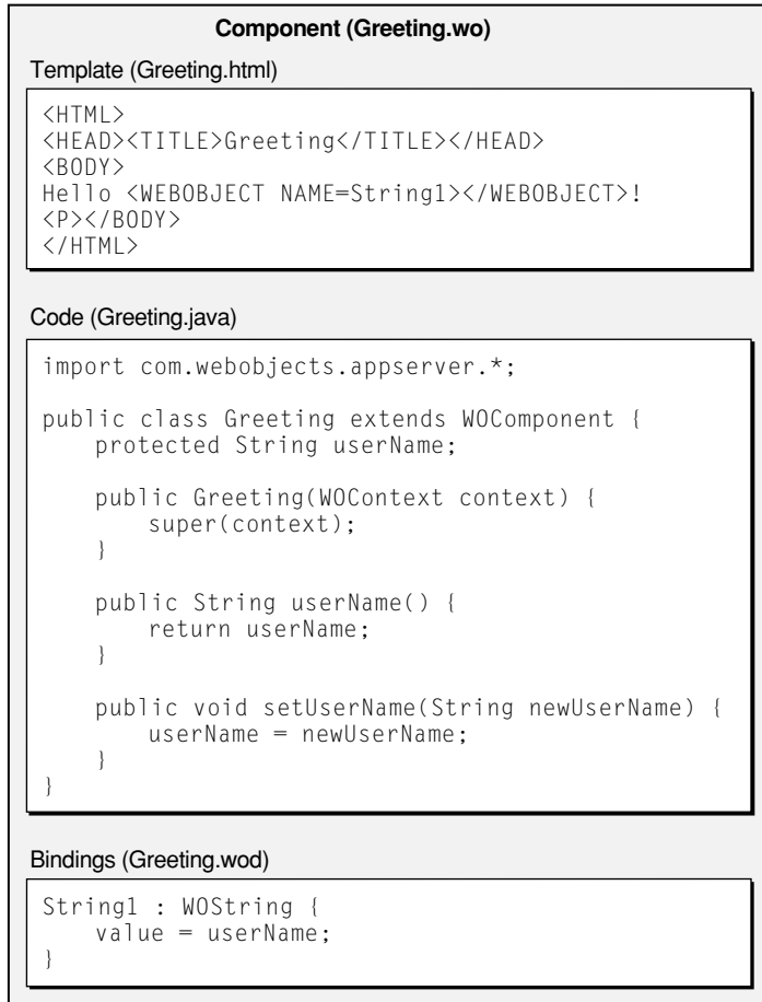
Figure 4-1 The files of a WebObjects component
