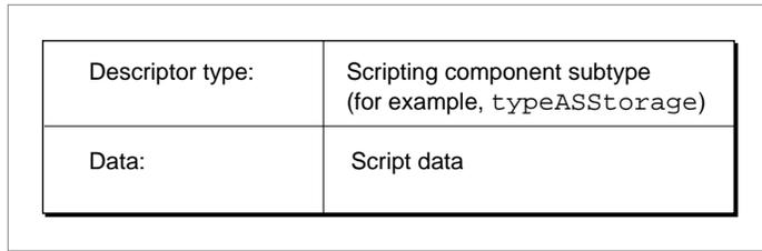
In most cases it is safest to request a handle to script data in the form of a generic storage descriptor record, regardless of the scripting component subtype you pass to the `OSASStore` function.
