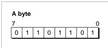
The base-10 value 109 is equivalent to the binary value 01101101. This sequence of binary digits exactly corresponds to the status of each bit in the byte illustrated in Figure 3-1. A byte value is typically represented by two hexadecimal digits. The value in Figure 3-1, for example, is equivalent to \$6D.
