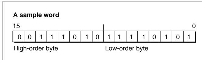
Using the word in Figure 3-8, the call `BitTst(myPtr, 0)` returns `FALSE` because bit number 0 in the first byte is not set. But the call `BitTst(myPtr, 11)` returns `TRUE` because bit number 3 in the second byte is set.
