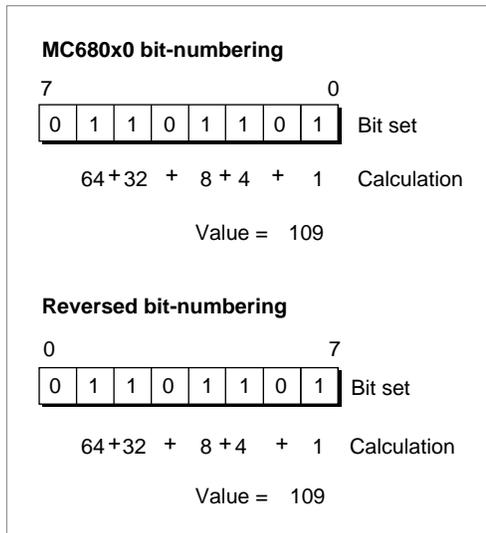
When using routines other than the `BitTst`, `BitSet`, and `BitClr` routines or if you are an assembly-language programmer, you should use the MC680x0 bit-numbering scheme.
