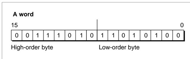
In Figure 3-2, the high-order byte is set to \$3A. The low-order byte is set to \$D4. The word thus has the value \$3AD4.
