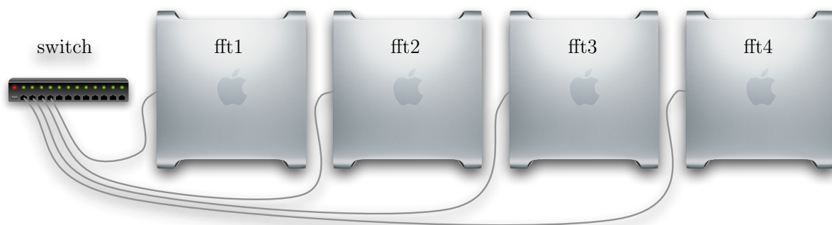
Figure 5: Diagram of the “canonical cluster.” This cluster consists of four PowerMac G5 computers, four Ethernet cables, an Ethernet switch, and four power cables. (Power cables not shown.)
