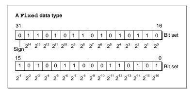
The high-order word consists of the integral component of the fixed-point number, and the low-order word consists of the fractional component of the fixed-point number. Each bit, other than the most significant bit, represents a power of 2, as indicated in Figure 3-5.
