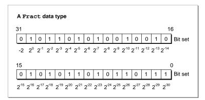
Like a Fixed number, a Fract number is a 32-bit quantity, but its implicit binary point is to the right of bit 30 of the number; that is, a Fract number has 2 integer bits and 30 fraction bits. As with the type Fixed, a number is negated by taking its two's complement. Thus, Fract values range between -2 and  $2 - (2^{-30})$ , inclusive.
