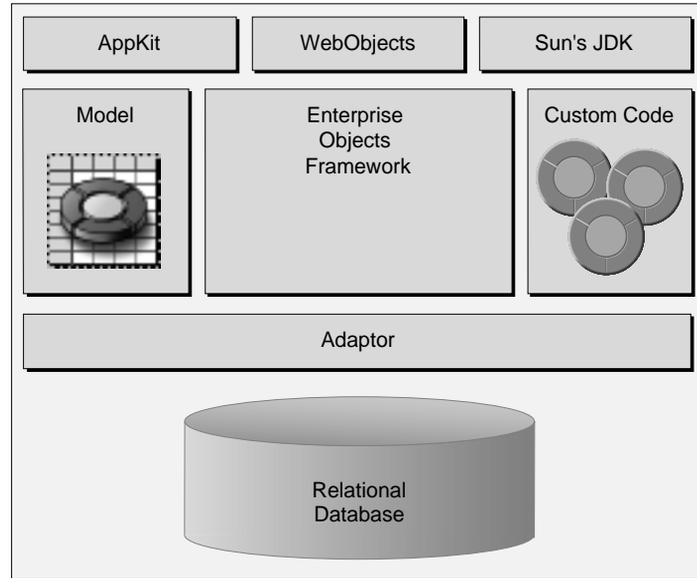
**Figure 6.** The Ingredients of an Enterprise Objects Framework Application
