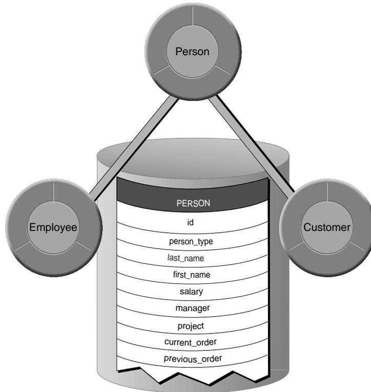
**Figure 30.** Single Table Mapping
