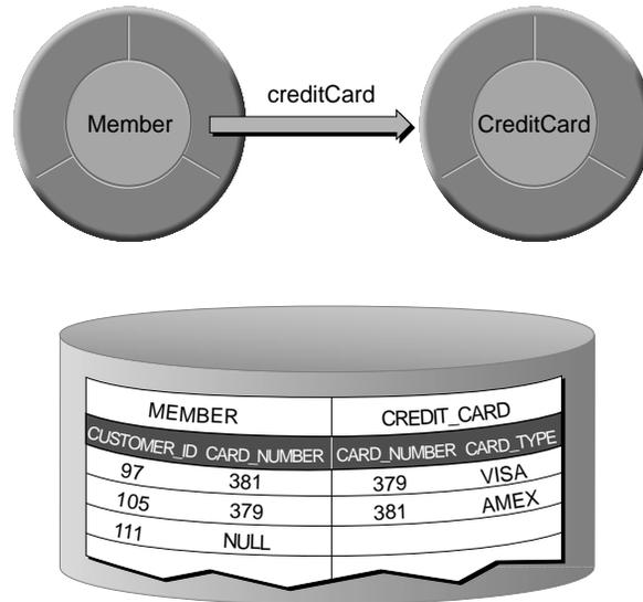
**Figure 24.** Storing a Foreign Key in the Source Table
