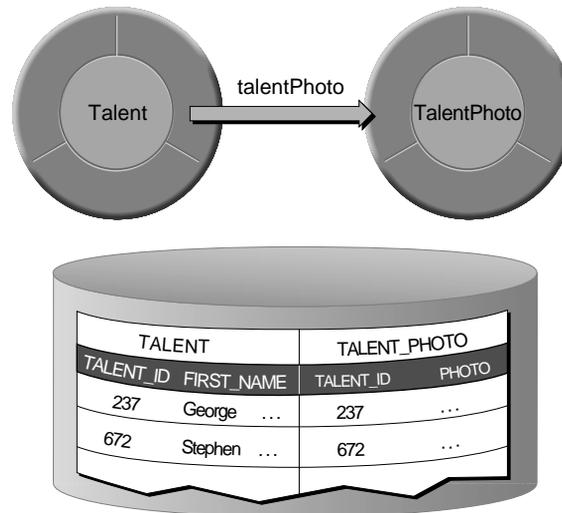
**Figure 25.** Storing a Foreign Key in the Destination Table
