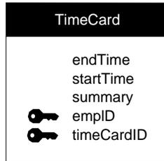
**Figure 56.** An Entity with a Compound Primary Key
