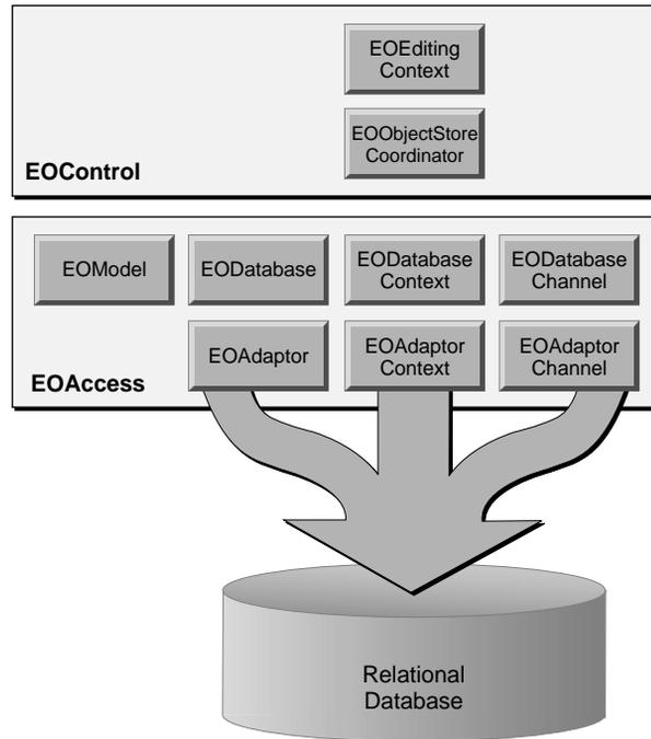
**Figure 11.** Framework classes in a Command-Line Program
