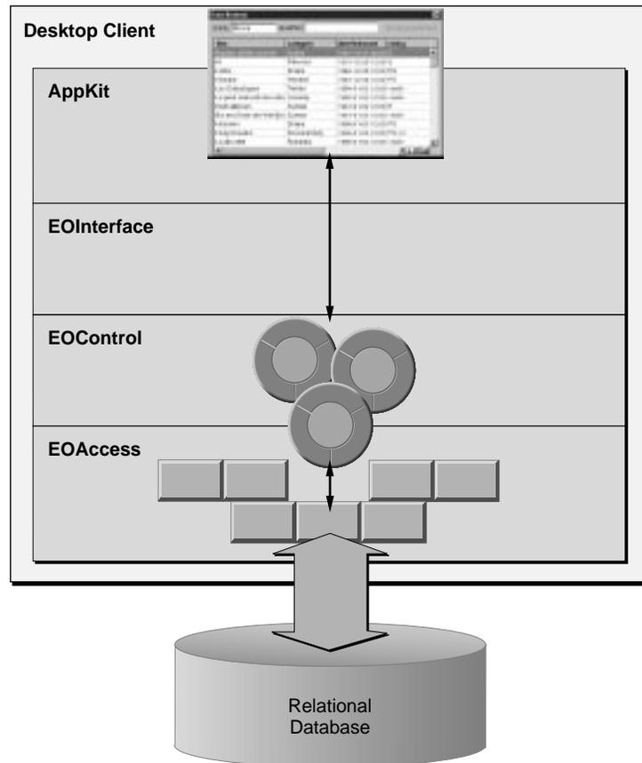
**Figure 8.** An Application Kit Client/Server Application
