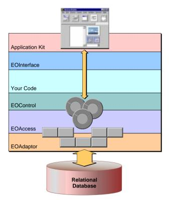
Figure 1. Architecture of Traditional Enterprise Objects Framework Application
