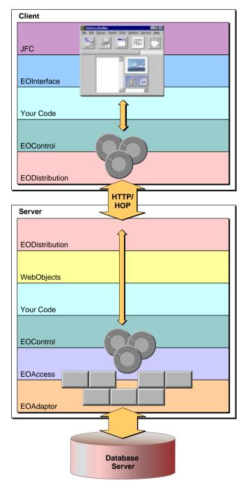
Figure 2. Architecture of Java Client
