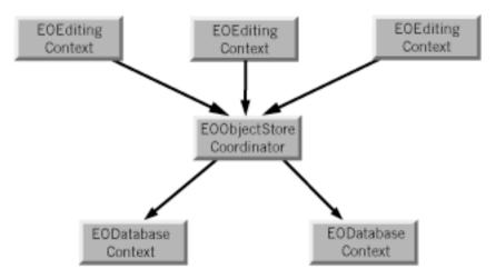
When an editing context fetches objects, the request is passed through the coordinator, which forwards it to the appropriate database context based on the fetch specification or global ID. When the database context receives a request to fetch or write information to the database, it tries to use one of its
