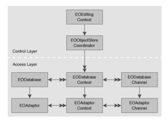
Figure 3 The EODatabase Level as an Intermediary Between the Adaptor Level and the Control Layer
