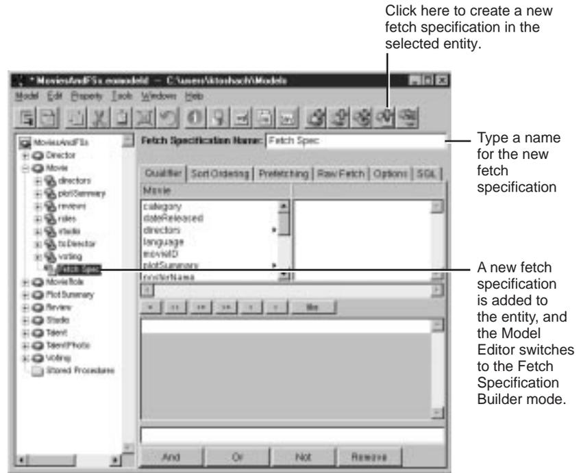
**Figure 40.** Adding a Fetch Specification to an Entity
