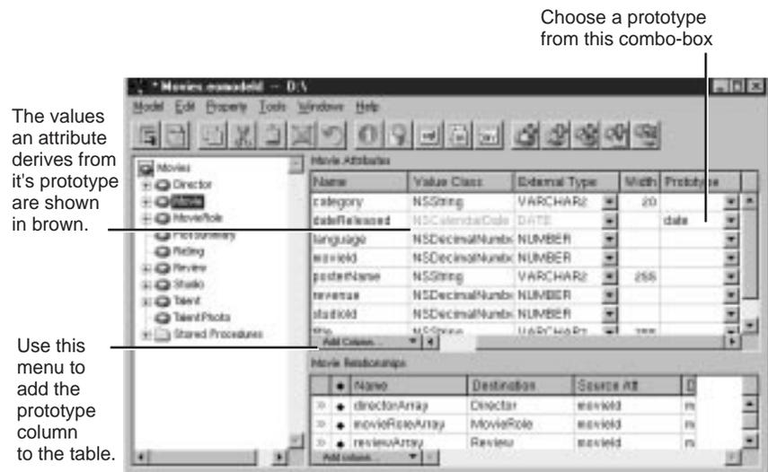
**Figure 22.** Assigning a Prototype to an Attribute
