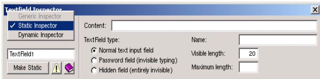
All WebObjects elements have a *dynamic inspector*, that is, one that allows you to set bindings (you'll work with bindings in the next section). In addition, many WebObjects elements (those with direct counterparts in static HTML) also have a *static inspector*. This inspector allows you to set the standard HTML attributes for that type of element.
