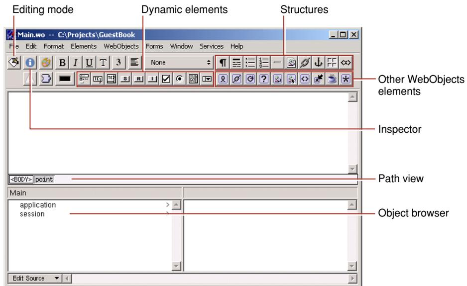
You create your component graphically in the upper pane of the component window. The browser at the bottom of the window (known as the *object browser*) is used to display variables and methods your component uses. Note that there are two variables already defined, `application` and `session`. You'll create others later.
