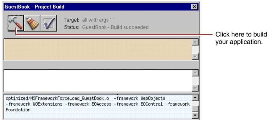
The Project Build panel displays the commands that are being executed to build your project. If all goes well, it displays the status message “Build succeeded.”
