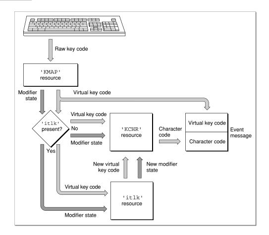
When a user presses or releases a key on the keyboard, the keyboard generates a raw key code. The system software uses a 'KMAP' resource to map the raw key code to a hardware-independent virtual key code and to set bits indicating the state of the modifier keys. A 'KMAP' resource specifies the physical arrangement of a particular keyboard and indicates the virtual key codes that correspond to each physical key.
