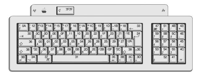
Figure 2-10 shows the virtual key codes as specified by the 'KMAP' resource for the Apple Extended Keyboard II, one that uses the Domestic (ANSI) layout, and one that uses the ISO layout. The labels for the keys on the ISO keyboard are shown using the French keyboard layout. The virtual key codes are shown in hexadecimal.
