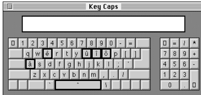
Figure C-14 Key Caps display of completer keys after circumflex dead key has been pressed
